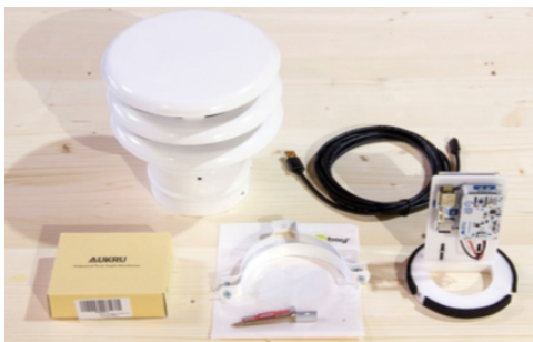
Figure 1 Citizen Kit with Prototype Enclosure
