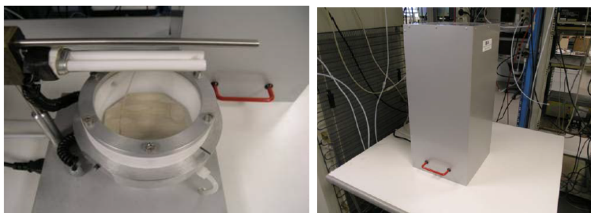
Figure 7: Laboratory test bench, with below the chamber tiles exposure (below left) and the chamber of the measuring sensors (below right).
