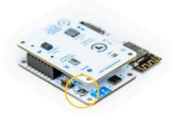
You can also perform a reboot by disconnecting the battery and the USB cable so that the kit is restarted. In this way we will not lose any data and configuration except the time in case of being in **SD mode**.
