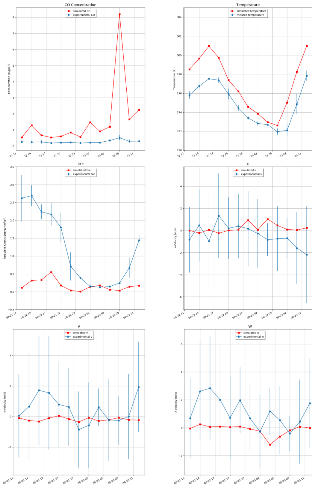
Figure 9 Marconi street, summer. Comparison between numerical results (red) and experimental results (blue). The uncertainty bars refer to the analytical uncertainty of meteorological and air quality observations.
