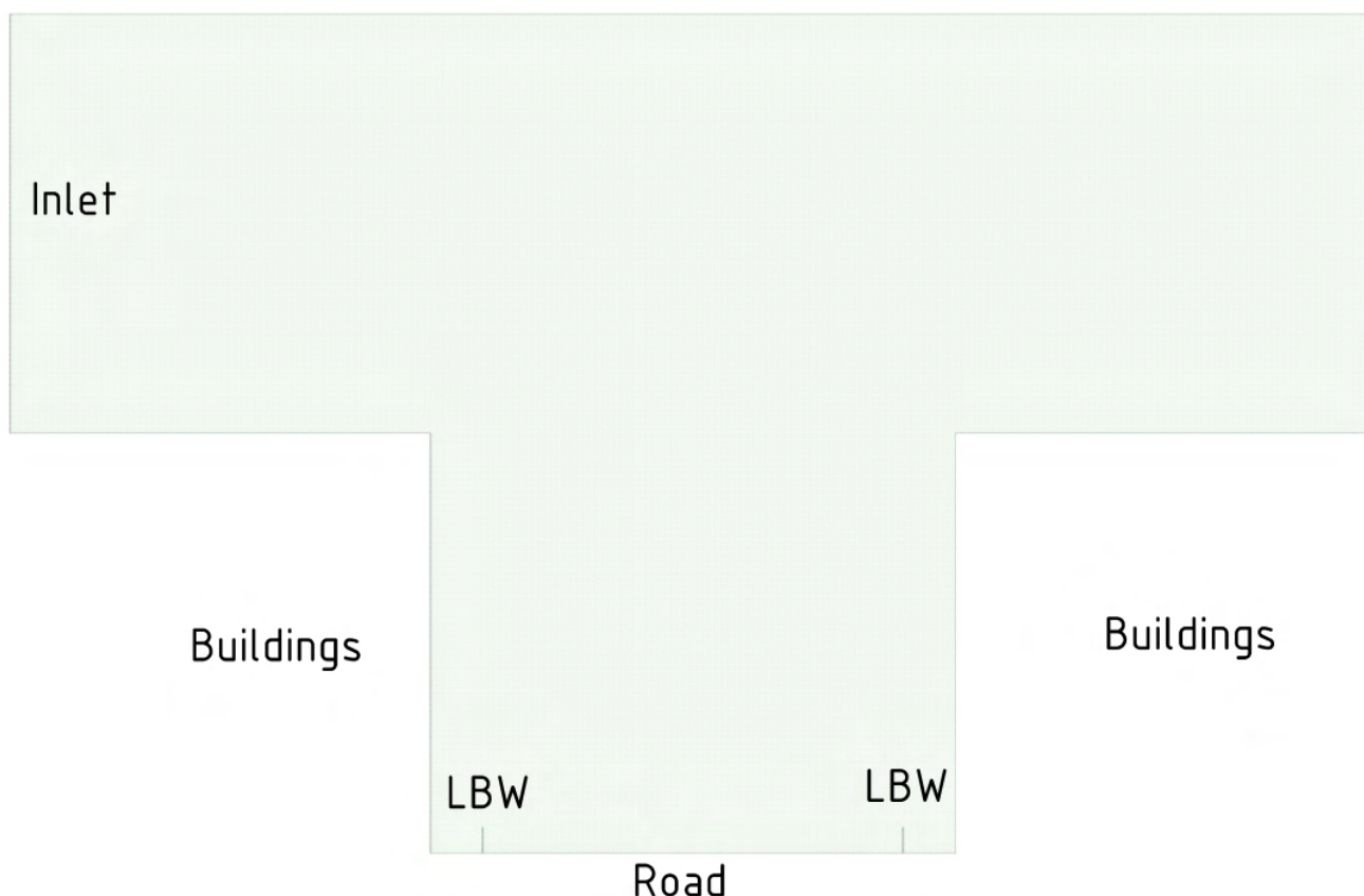
Figure 101. Cross-section of the canyon at Pearse Street showing locations of low boundary walls (LBWs).
