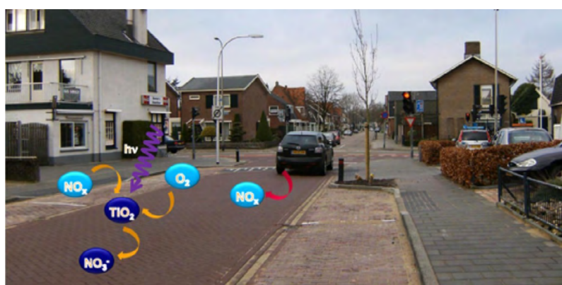
Figure 3: Air purifying pavement to reduce NO x concentration in Hengelo, Netherlands. (Source: Ballari, M.M. and Brouwers, H.J.H., 2013. Full scale demonstration of air-purifying pavement. Journal of Hazardous Materials , 254-255, 406-414)
