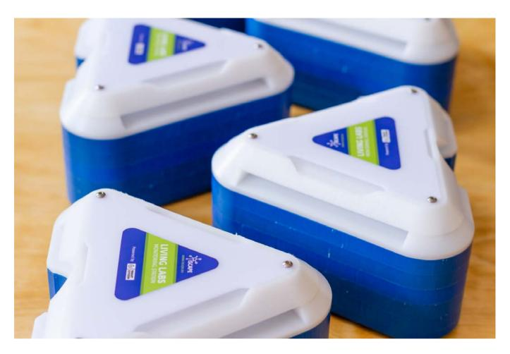
The station is designed with a modular principle where sensors can be added easily added expanding the capabilities of the installation or replaced when they are damaged or the sensors lifetime is over. From a costs perspective while being more expensive than the Smart Citizen Kit it is also conceived as a low-cost solution.
