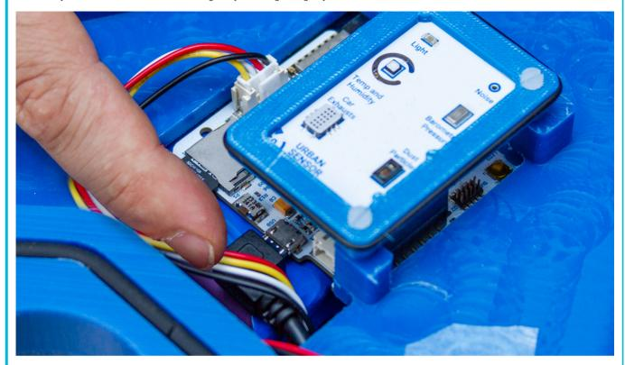
After 5 seconds the light will go off and will go on again after 15 seconds. Then you can release the button and your device will be fully resetted as a brand new Station.
