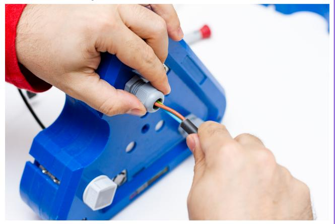
$\boldsymbol{\cdot}$  Cover the cable gland again and remove the square cable gland on the other side
