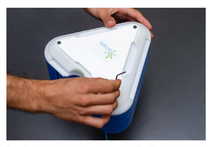
Then turn off your Kit by pressing the button for **5 seconds** and remove the micro SD card. You can plug the card on your computer using a Micro SD card reader.
