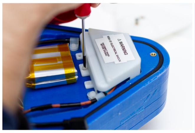
• Make sure there is no energy left in the power supply by checking that there is no LED on in it. Then, remove the cables from the power supply and the white brackets
