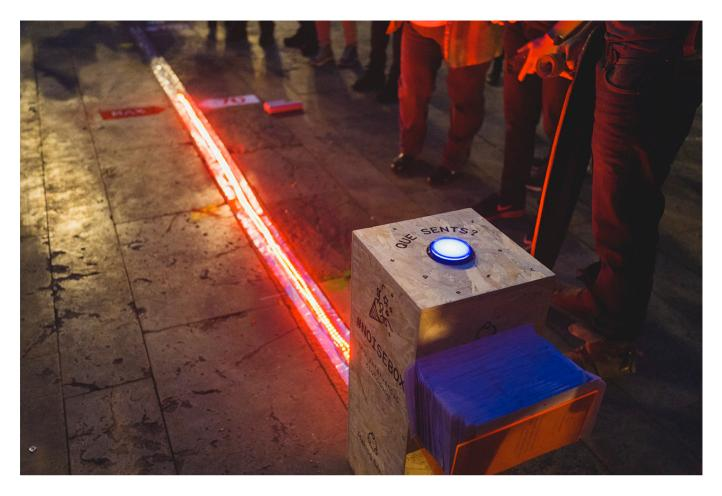
The device comprises a wooden box equipped with a Smart Citizen Kit to which was a 5 meter long LED strip has been attached. Participants can press a button on the box to trigger the noise sensor. The original installation was battery powered but it can also be plugged to simplify the design and cost.
