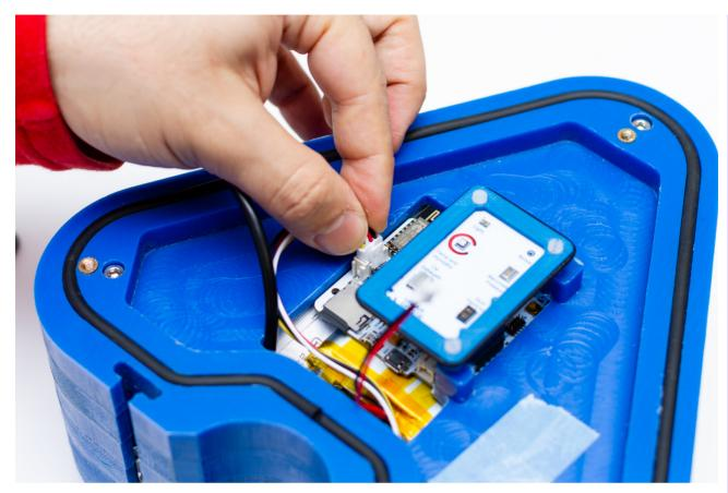
• Put the kit's layer on again. Verify that the o-ring fit's in properly. Close everything and put both layers back on on
