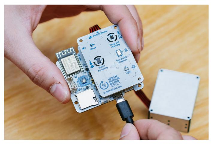
The first step is to connect the battery. The kit will light in red (configuration mode) and we will be able to configure it by following the instructions at start.smartcitizen.me.
