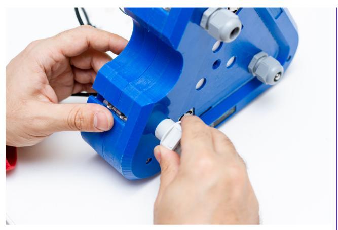
• Exchange the rubber in the cable gland with the one provided with a hole
