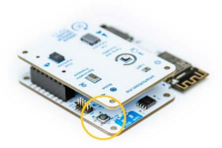
You can also perform a reboot by disconnecting the battery and the USB cable so that the station is restarted. In this way we will not lose any data and configuration except the time in case of being in **SD mode**.
