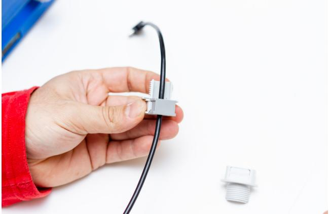
• Put the cable in and fix the gland in place. Leave sufficient overhead in the cable to be able to connect it to the kit
