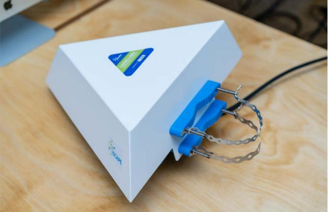
• Put the station in it's final location, and tighten it with the perforated steel stripes. Play with both sides, so that the stripes are tight on the pole
